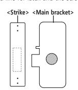
Mark the location for perforation and screw for latch and main bracket.
